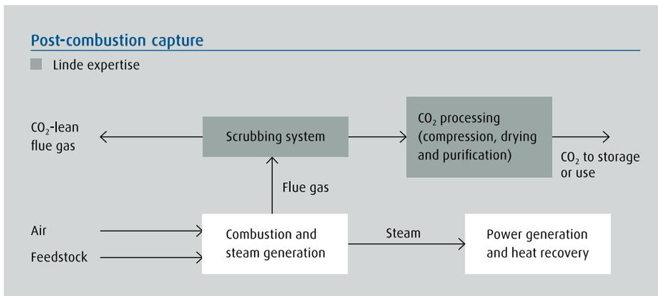
In post-combustion capture, CO<sub>2</sub> is separated from the flue gas by scrubbing, using a chemical solvent such as amine.
