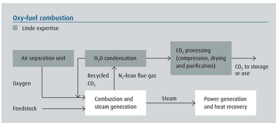
In oxy-fuel combustion, the fuel is combusted with oxygen and recycled CO<sub>2</sub>-rich flue gas. Oxygen is used instead of air to reduce the nitrogen concentration in the flue gas. This allows for the cost-effective recovery of CO<sub>2</sub> from the flue gas.
