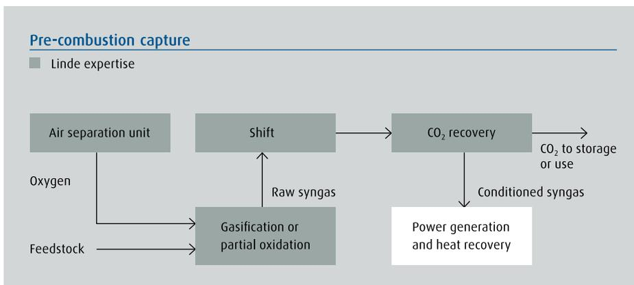
In pre-combustion capture, also known as IGCC (Integrated Gasification Combined Cycle), the fuel is first gasified with oxygen to produce a synthesis gas. This gas is then chemically converted into separate streams of carbon dioxide and hydrogen in the so-called shift reaction ( $\text{CO} + \text{H}_2\text{O} \rightleftharpoons \text{CO}_2 + \text{H}_2$ ).
